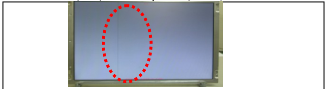
Fig. 2 – Vertical line defect in TFT-LCD panel.
